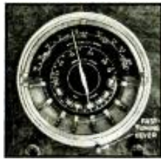
Close-up of Flash-Tuning dial. (When a station tuning tab has been reached) close the flash-tuning circuit.
