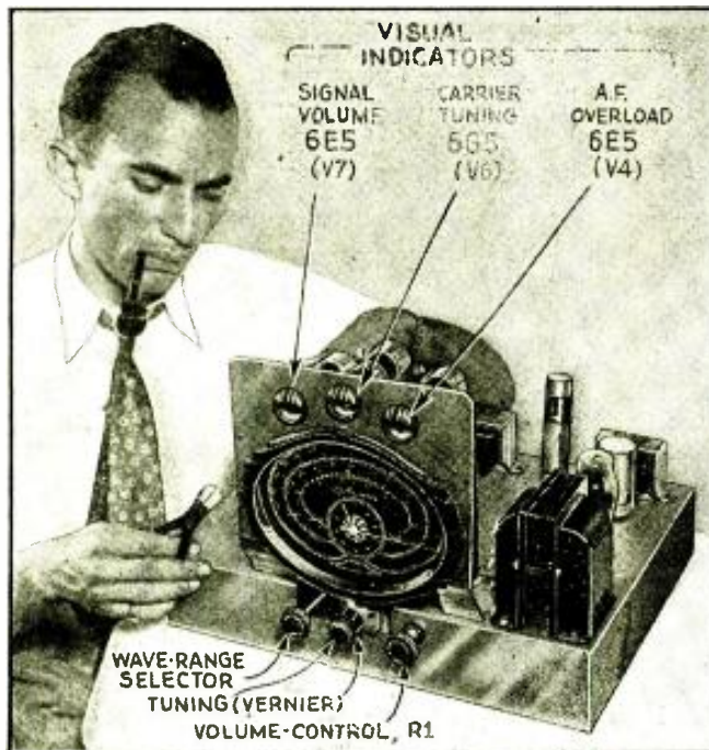
Fig. B. The R.F. all-wave tuner (Chassis No. 1) of the 30-Tube Set.
