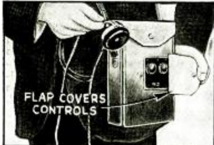
Fig. B. Portable battery radio set in camera case.
