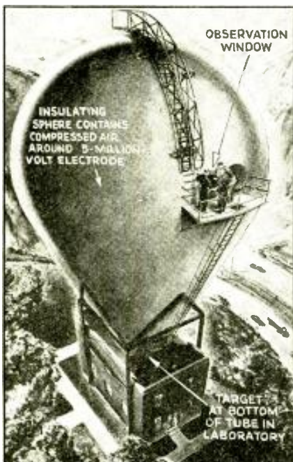
Design of the new "atom-smashing" tower to be erected by Westinghouse at East Pittsburgh. Inside the 30-foot globe is an electrode charged to 5,000,000 volts, by the tension of which electric "bullets" are shot down on a target 35 feet below. By this means, discoveries of importance in radio and other branches of physics are expected.
